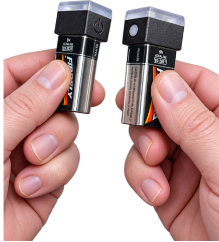
Figure 1. The white-dot magnet and the power-symbol reed switch.
